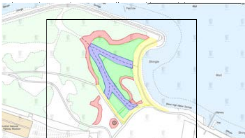
Figure 2. Original proposed design of the meadow; green- area to be sown; blue- pathways through the meadow; red- areas to be potentially plug planted and left uncut (only one of these was selected in the bottom right of the plan).
